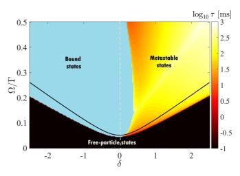
FIG. 6. Stability diagram around the equilibrium point  $r \approx \lambda$  for  $\ell = 0.09$ . Free-particle states are found for low pump intensity (black region), bound states on the red-detuned side (light blue), and metastable states in the blue-detuned side, where the color gradient denotes the state lifetime. Simulations realized with particles with an initial temperature  $T = 1 \mu K$ , where the conversion between temperature and velocity was realized using the Rb atom mass.
