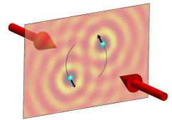
FIG. 1. Two atoms evolve in the z = 0 plane, trapped in 2D by counterpropagating plane waves, with the wave vector orthogonal to that plane. The light exchange between the atoms induces the 2D two-body optically coupled dynamics.
