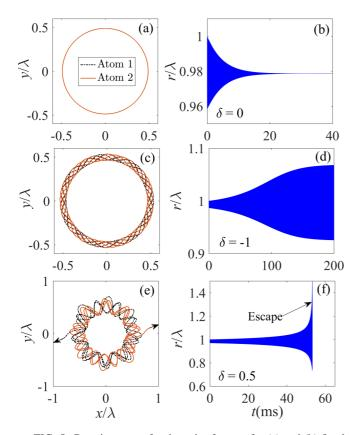
FIG. 5. Rotating states for the pair of atoms for (a) and (b) fixed interparticle distance, (c) and (d) vibrational mode, and (e) and (f) metastable state. As the orbits of both atoms coincide in (a), only a single orbit is displayed. Simulations realized with  $\ell = 0.09$ ,  $\Omega/\Gamma = 0.25$ , and  $T = 1 \mu$ K, where the <sup>87</sup>Rb atom mass was adopted.
